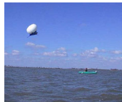
Picture 4. 2.0 cu metre Helikite flying from a 11ft dinghy in Mexico, to lift a video camera.
