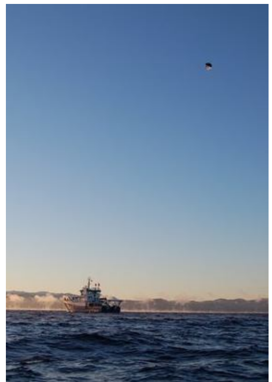
Picture 8. Helikite flying from research vessel to provide long-range USV relay.
