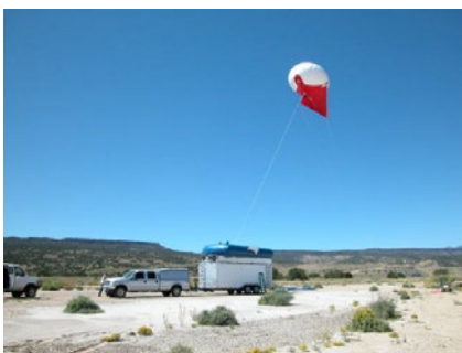
Picture 5. Thirty four cubic metre Skyhook Helikite deployed to 1500ft within 20 minutes in all-weather.
