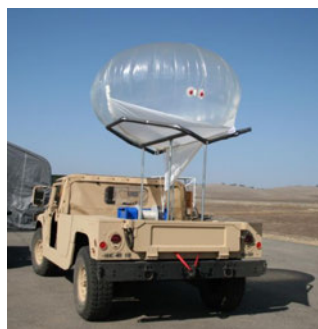
Picture 6. Three cubic metre Stealth Helikites deployed on HUMVEES in California.
