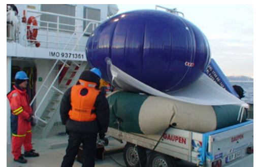
Picture 7. Six cubic metre Helikite ready to launch from a Helibase placed on the stern of an arctic research vessel.
