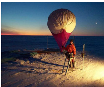
Picture 2. Three cubic metre Skyhook Helikite operating from a hole dug into the ice in Antarctica.
