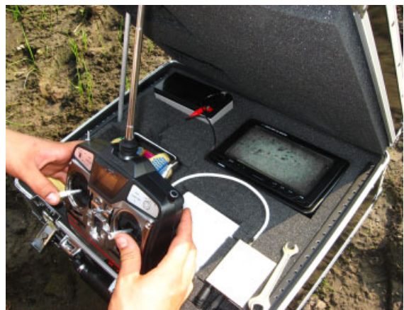
Figure 6. Steering the digital still camera by assistance of the live video link (photograph by W. Gheyle).
