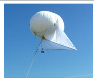
34m3 Helikite steadily lifting E/O + I/R Gyro-Stabilised military surveillance camera.
