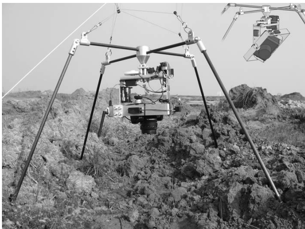
Figure 7 The cradle with mounted camera
