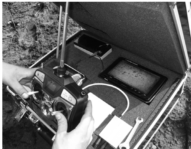
Figure 8 Steering the camera by assistance of the video live link
