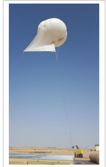
34m 3 Helikite steadily lifting E/O + I/R Gyro-Stabilised military surveillance camera.
