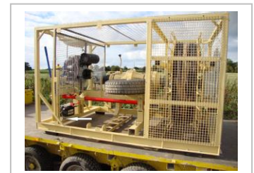
The Rapid-Reaction trailer can inflate, launch and then tow the high altitude Helikite very steadily at speeds up to 30 mph.
